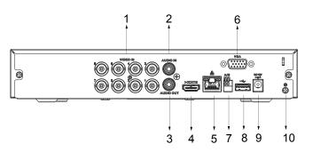
1 Video In 2 Audio In 3 Audio Out 4 HDMI Port 5 Network Port 6 VGA Port 7 RS-485 Port 8 USB Port 9 DC 12V Power Input 10 Ground
